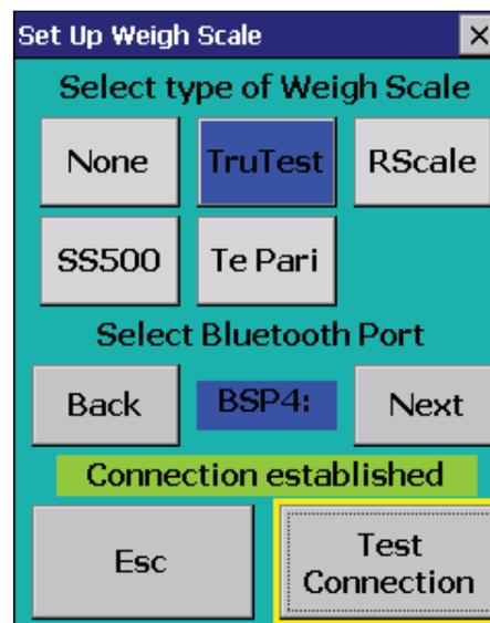
6. Tap **Test Connection**. The message **Connection Established** means the stock recorder and your weigh scale have been successfully connected. Press **Esc** to exit.
