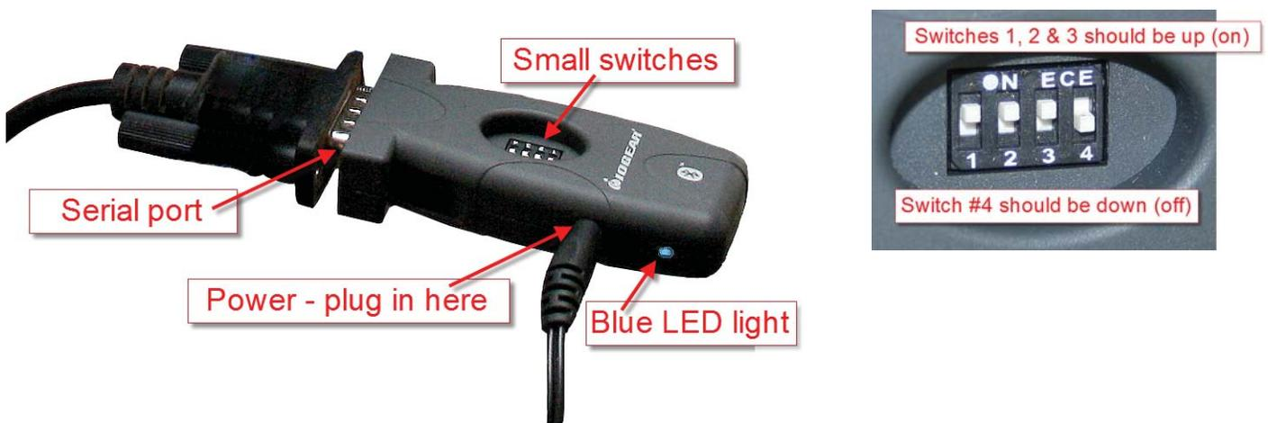
5. When the blue light is blinking once every 2-3 seconds it is in "discovery mode". This means it is ready to accept a Bluetooth connection.
